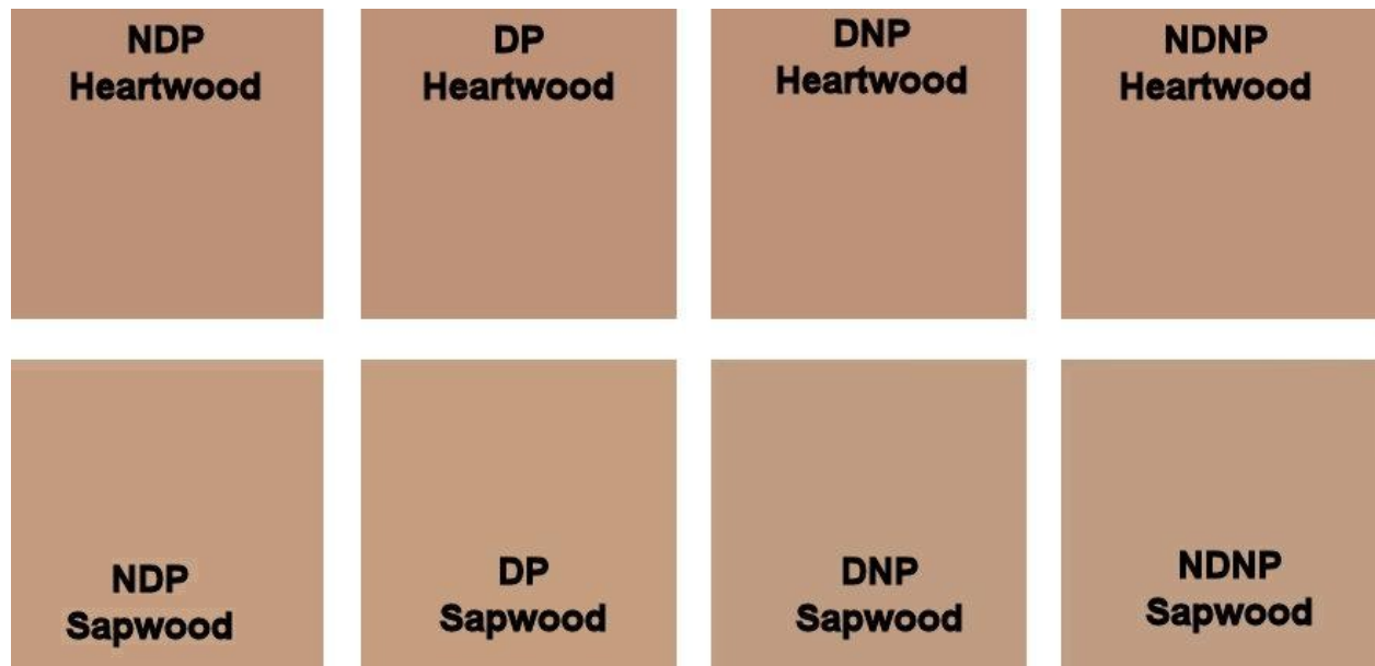
Figure 8. Average color readings for heartwood and sapwood of NDP, DP, DNP, and NDNP lumber
