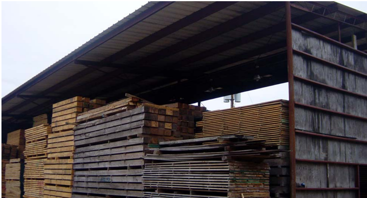
Figure 4. Air drying shed with ceiling fans to ensure continuous airflow
